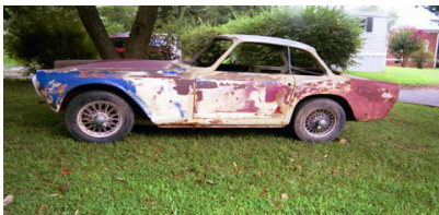
Italias were all steel bodies, and while sturdy, tend to rust when left outdoors. Stoner hopes to rebuild both cars.
